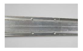
4. Snap the ReductoClip furring channel into the ReductoClip by squeezing the furring. IMPORTANT: Make sure to overlap channels by 150mm and secure with 4 self tapping screws (not supplied). Make sure overlaps occur between the clips, not on the clips. Ensure furring channels are overlapped alternatively, front to back and so on.
